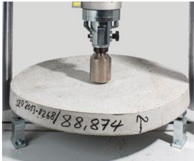
Round panel test: ASTM C1550
