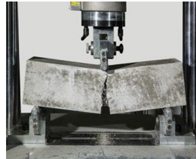
Beam test: EN 14651
